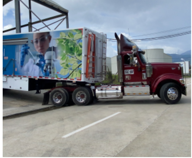
Full lateral view of the unit showing the complete truck-semitrailer assembly. The 15-meter overall length accommodates all functional laboratory zones without compromising mobility on secondary roads.
